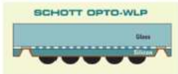
Opto wafer level CSP with tapered TSV interconnection
