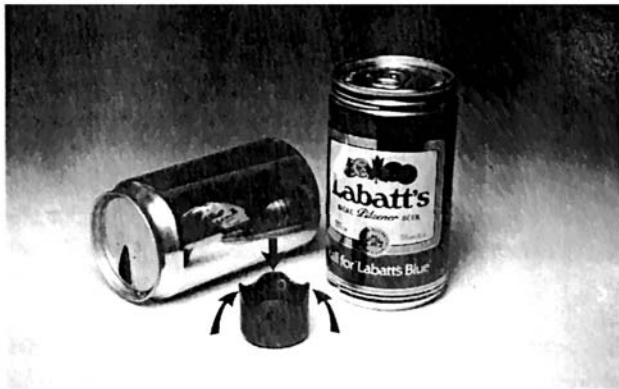
Figure 3. Aluminium beverage cans. On the small sample, ears are marked by arrows.
