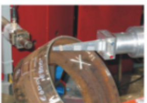
BT-8 residual stress measurement rig. Hoop stress
